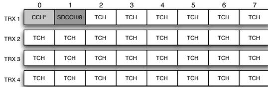
**Figure 4: An example air interface with four carriers (each showing a single frame). The first time slot of the first carrier is the Common CCH. The second time slot of the first channel is reserved for SDCCH connections. Over the course of a multiframe, capacity for eight users is allotted. The remaining time slots across all carriers are designated for voice data. This setup is common in many urban areas.**
