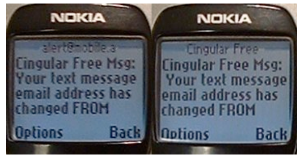
Figure 6: Spoofing a service provider notification is trivial due to interface and message length constraints; the left image is a forgery of a legitimate service notification (right) provided by Cingular (Note the top line).
