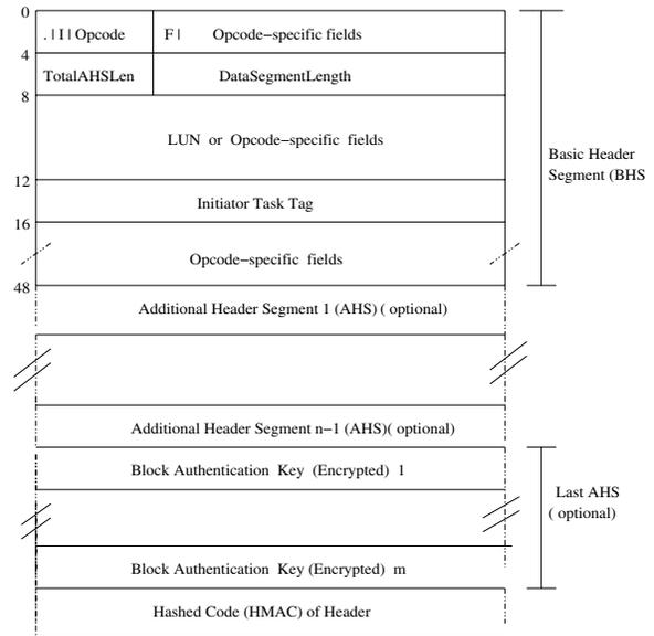
**Figure 5: Modified Format of iSCSI PDU header for Lazy Authentication. The Block Authentication keys are encrypted using the secret IPsec key and sent in the AHS. They are followed by the HMAC of the header.**
